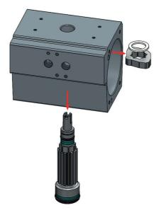
Fig.10 - Pinion removal
