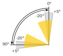
Version with extended angle of rotation adjustment (new version) from GD-040 to GS-160 Inner end position +5° to -20
