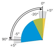
Version as combination cover screw with extended angle of rotation adjustment from GD-052 to GS-160 Inner end position -5° to +20
