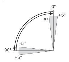
**Standard version** from GD-040 to GS-400 Inner end position -5° to +5° Outer end position +85° to +95 Type code example: GD-092/090-F03/F05-V11-F
