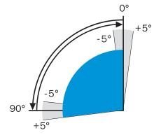
**Version with cover screw** from GD-052 to GS-210 Inner end position -5° to +5 Outer end position 0° to +95° for 90° actuators Type code example: GD-092/090-F03/F05-V11-F-**OA Designation -OA = O**uter **A**djustment
