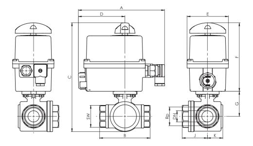
Fig. 13-4 Dimensional drawing Type EKT (exemplary representation with ER Plus rotary actuator)
