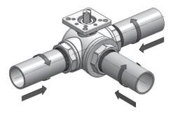
Fig. 5-1 Mounting a ball valve in pipeline
