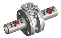
Fig. 5-1 Mounting a ball valve in pipeline
