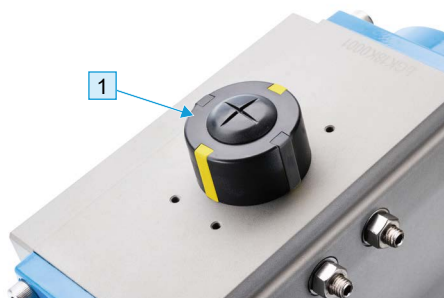
Fig. 3-12 Operating and display elements of the rotary actuator bar-agturn Longitudinal design = open position Transverse design = closed position
