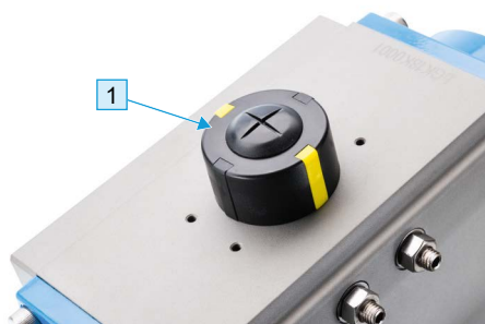
Fig. 3-11 Operating and display elements of the rotary actuator bar-agturn Longitudinal design = closed position Transverse design = open position
